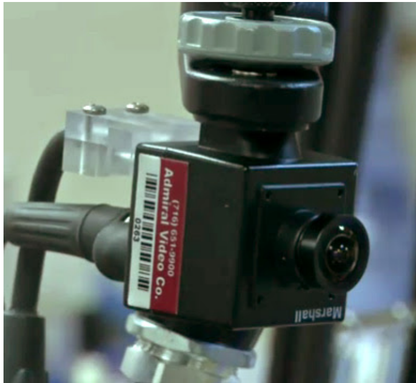
The pylon cams are based on Marshall POV units.
