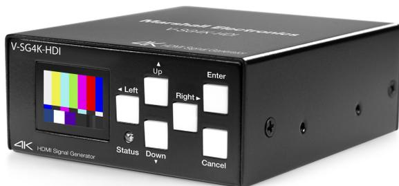
The TITAN V-SG4K-HDI is capable of generating nearly any combination of display resolutions, sampling and frame rates in the digital spectrum, along with an extensive array of audio combinations. The device generates audio tones from two to eight channels, 16 to 48-bits, and 32-192KHz sample rates. The audio jack allows insertion of audio from external source (two channels).
