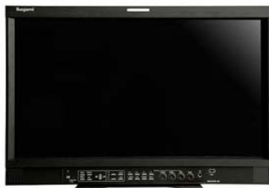
The Ikegami HEM-2570W is a 24.5-inch, grade-1 OLED HD monitor with built-in audio functions, such as speakers and headphone terminal, as well as 3G-SDI, Multi-SDI, DVI-D, VBS inputs.
