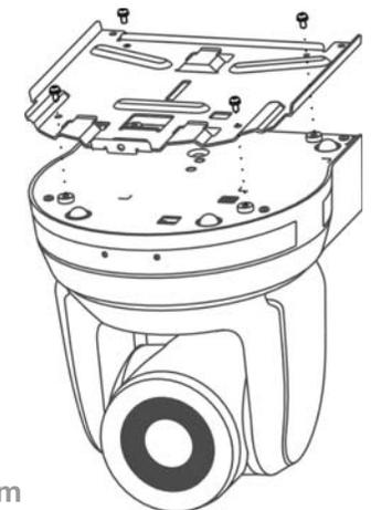
3. Lock the metal plate B on ceiling mounted hanger
