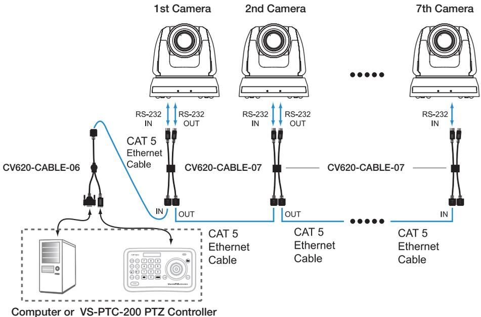
\* The CV620-CABLE-06 cannot be connected with a Computer and a VS-PTC-200 Controller at the same time
